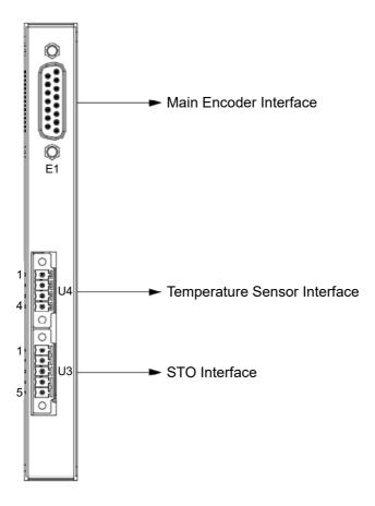
The control platform of AxN-DC drive supports SinCos encoder, Endat 2.2 encoder, Resolver, digital incremental encoder, Nikon encoder and, Tamagawa absolute encoder and Hiperface encoder.
