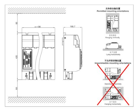
1) For proper air circulation, at least 60 mm clearance must be available above and below the module.
