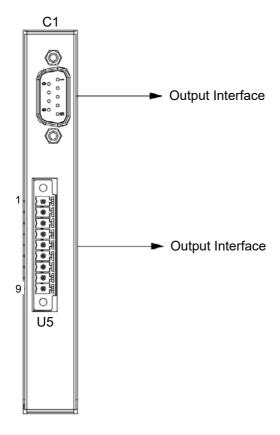
Interface and Wiring Auxiliary Encoder Card
