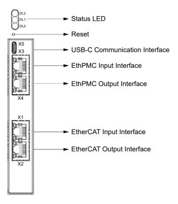
Interface and Wiring CPU Card
